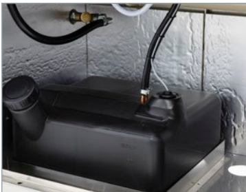
31LT EASY FILL INTERNAL FUEL TANK
